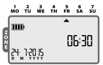
In **AUTO RUN** mode, the WPX will irrigate each zone per its programmed schedule. If any zones are scheduled to run at the same time and day, your controller will place those zones in a queue and irrigate one valve at a time, starting with the lowered number zone first.
