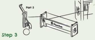
Attach the polystyrene float to the float indicator and slot into arooves inside the trough.
